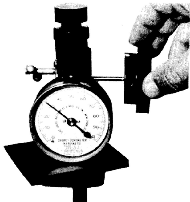
Figure 8. Durometer testing of neoprene rubber.
