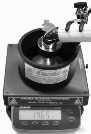
Front view of the PUP-50. Shown is the electronic balance, base assembly, and test tank.
